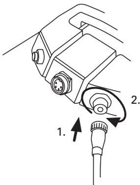
The connector at the end of the module cable is put into the battery charging plug and secured for water-tightness.
