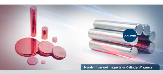
They represent a popular shape of Rare earth magnets and perment magnets. Rod magnets have a magnetic length which is larger than their diameter. This enables the magnets to generate very high levels of magnetism from a relatively small surface pole area. These magnets have high ,Gauss' values because of their greater magnetic lengths and deep depth of field, making them ideal for activating reed switches, Hall Effect sensors in security and counting applications.
