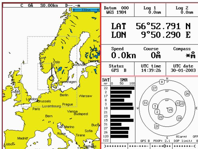
The displays, which are not related to the chart function, can be exchanged with a different one. It is also possible to change the right half of the screen from two quarter windows to half screen window, and vice versa. See section 2.1.2 how you go about changing the displays.
