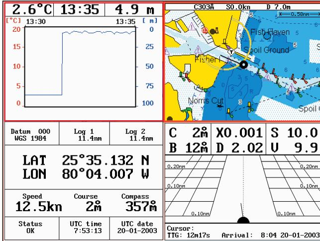
The displays, which are not related to the Echo function i.e. all displays except the Depth & temperature diagram in the top left quarter of the screen, can be exchanged with a different one. It is also possible to change the right half of the screen from two quarter windows to half screen window, and vice versa. See section 2.1.2. how you go about changing the displays.
