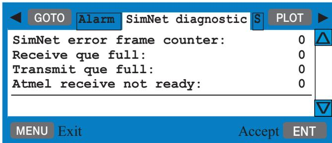
**SimNet error frame counter** - if the figure is not 0 it could be due to a number of things and not necessarily that there is a system error. However, if the counter is active and the number is rapidly increasing, then the system has detected a fault.
