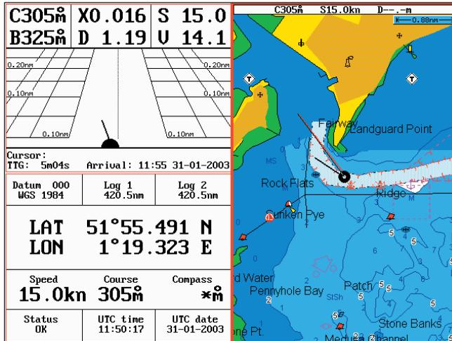
The displays presented in the example above are the default displays for Custom screen 1 under the PILOT menu.
