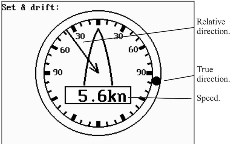
The Set & Drift display will show how fast the current is moving in knots; in what direction (true) it is moving and what direction in relation to the vessel (relative).
