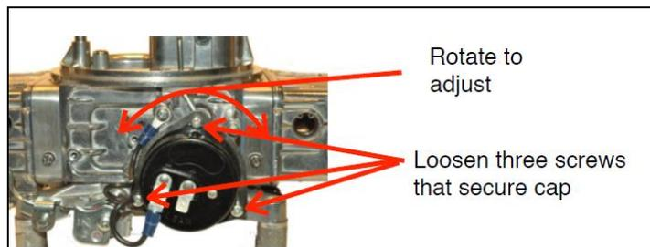
Clockwise rotation reduces temperature for choke to close and shortens the time for the choke plate to completely open. Full clockwise rotation the choke will never close. Counter-clockwise rotation raises the temperature for the choke to close and lengthen the time the choke plate is closed, so it will take longer for the choke plate to open to full vertical position.
