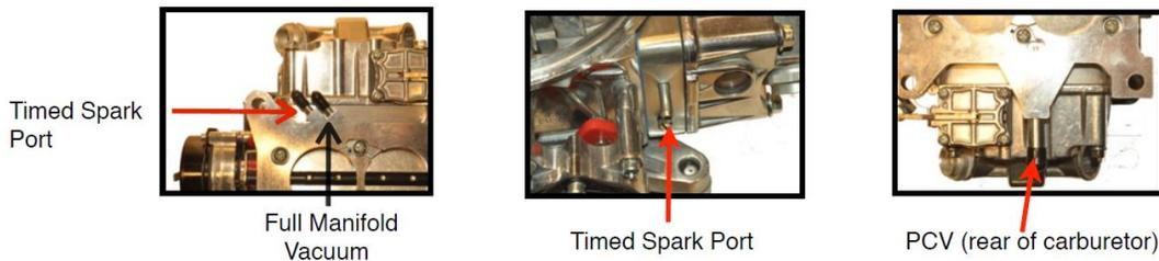
Distributor vacuum advance may also be connected to the tube in the primary metering block.
