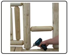
6) Insert Screw in side of the back where inserts into seat. Repeat on the other Back Assembly.
