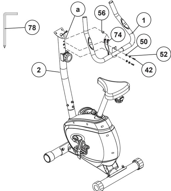
**STEP 6****Installation of the computer (14) at handlebar support (2).**
