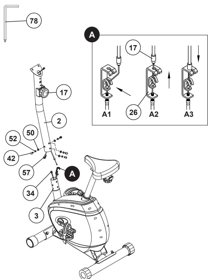
**STEP 5****Installation of handlebar (1) at handlebar support (2).**
