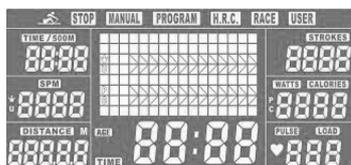
If no button are pressed and the pedals have not been moved for approx. 4 minutes, the computer will switch to power saving mode.
