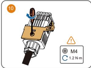
For inverter models  $\geq 15$  kW
