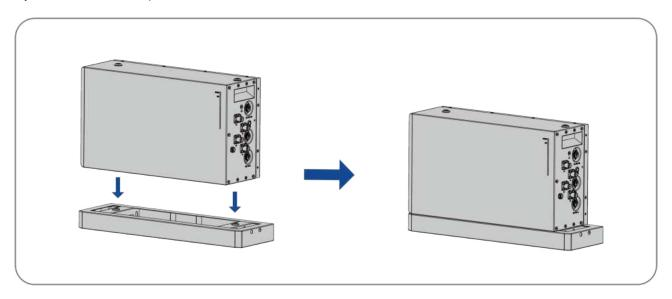
**Step 3:** Attach the right anti-tipping bracket by aligning the module locking plate (right) with the screw holes. Secure with four M5x10 screws, tightening to 4 Nm.
