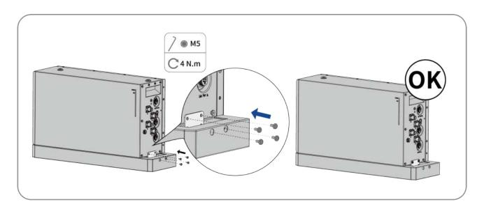
**Step 4:** Install the left anti-tipping bracket, using the module locking plate (left) to align the screw holes from above. Use four screws (M5x10) to secure the module lock plate (right), tightening torque :4 N.m.
