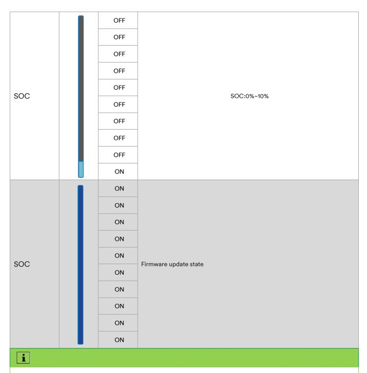
There are ten LEDs to indicate the State of Charge (SOC) of the battery and the different status of the LEDs indicates the different working state of the battery.
