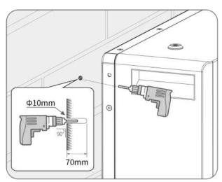
**Step 8:** Clean the dust from the hole, then insert the expansion bolt. Fix it with a rubber hammer, and tighten the nuts using a wrench. Next, fix the bolt tail and remove the nut, spring washer, and flat washer and reserve them for the next step. Repeat on the other side of the battery.
