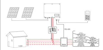
Note: As shown in the figure above, a switch must be installed at point A.In the process of use, if the SPH needs to be turned off, please turn off the switch at point A.
