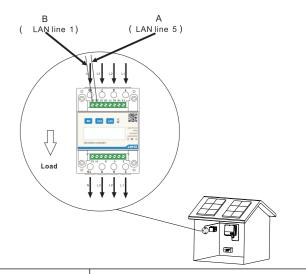
d. Connect the A+ (White-Blue)of Rs485 cable to Pin24 and B- (White-Orange)
