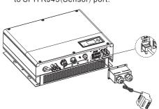
f. The standard RS485 cable length is 5m. If the length is not long enough, plaease add another cable to extend the length.
