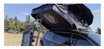
16.Hold the bottom of the ladder and lift the ladder forcefully so that the top of the ladder moves towards the tent.
