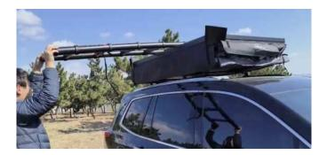
10. Push the ladder down as far as possible. In this way, lift the tent up perpendicularly.
