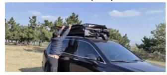
18. Tuck the exposed fabric around into the roof tent.
