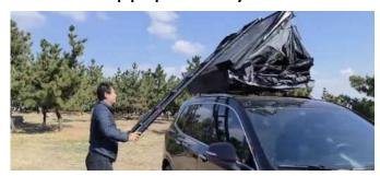
11. Pull the ladder so that the bottom moves in your direction.
