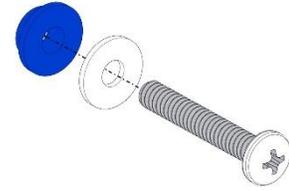
Assemble all 10-24 X 3/4" screws with one white and one blue washer. then install them in the vertical edges of the quarters dome. Keep the remaining 12 for the top of the dome.
