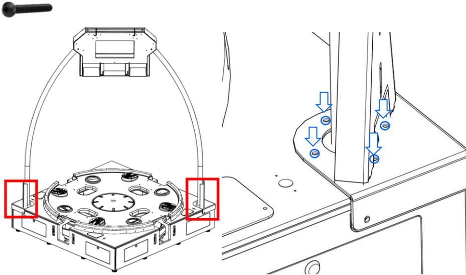
Secure each corner with the provided 2” button head screws and the ¼-20 locknuts
