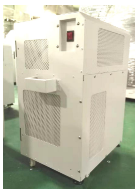
Right blower box
