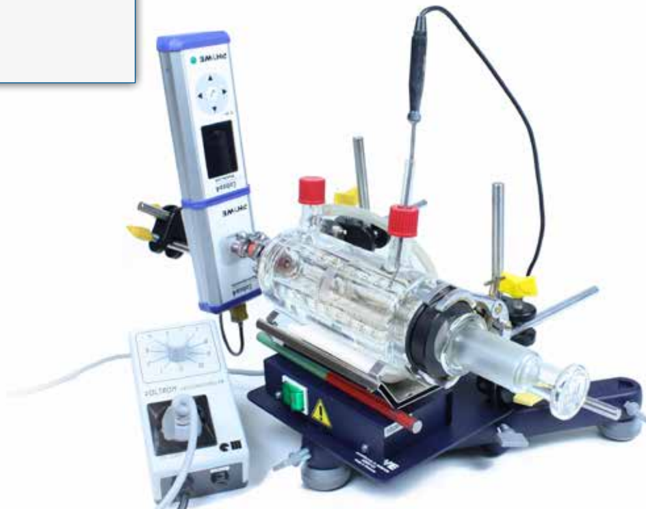
Correlation between volume and pressure under isothermal conditions.
