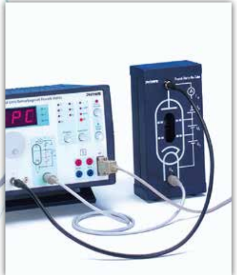
Franck-Hertz experiment with Ne-tube.
