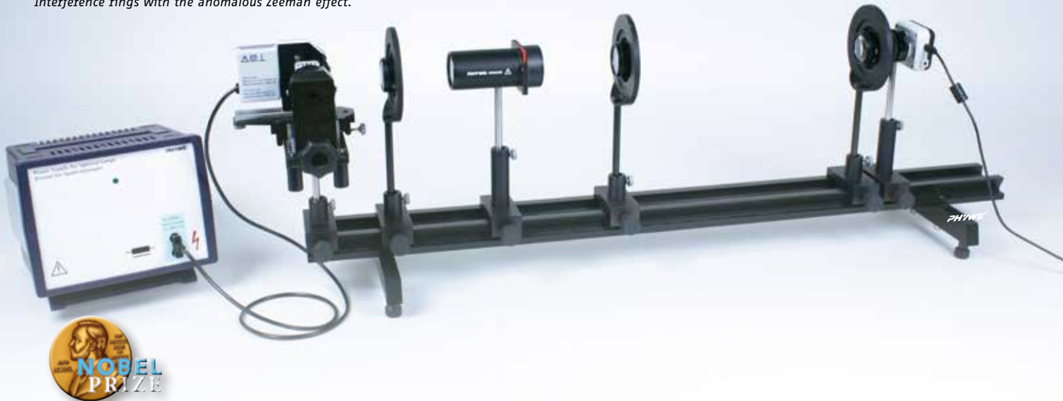
Interference rings with the anomalous Zeeman effect.
