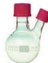
**Kolben, rund, 100 ml, 3 x GL 25**
