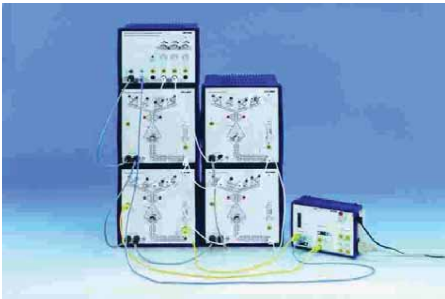
Experimental set-up to show direction selectivity by unilateral inhibition.
