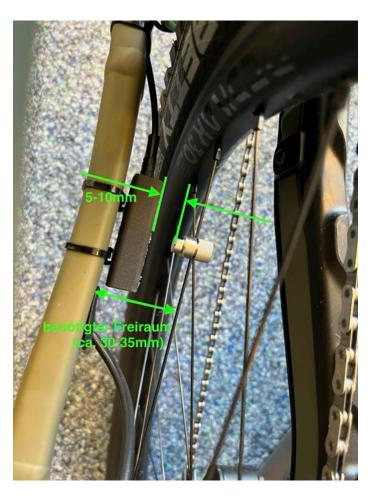
5) Now all that remains is to plug the pulse coil into the badassBox, then the badassBox can be coupled. (Turn over to the Boost Buddy-App)
