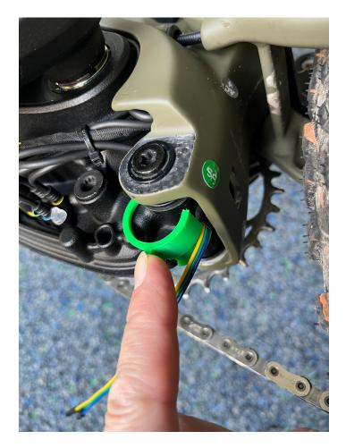
Without having to remove anything other than the motor protection cover, the pulser coil can be neatly installed in just a few steps and aligns itself.
