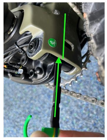
As soon as the semicircular surround is in contact with the bulge in the motor housing, push the complete pulse generator unit fully on by pressing lightly on the small handle bar (only Rim 38 type, on Rim 37 just push on the same point).
