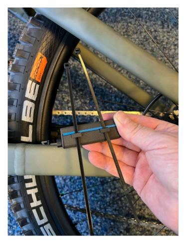
The exact position is largely irrelevant, the only important thing is that there is sufficient clearance (approx. 30-35 mm as shown in the picture) between chainstay and the spokes.
