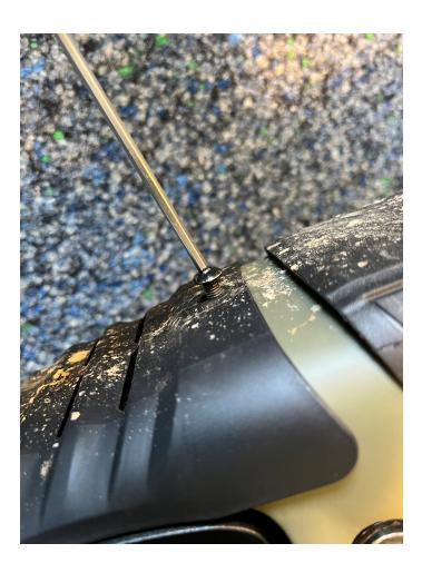
2) The excitation coil is installed at the rear end of the motor. To do this, it is inserted on the left (in direction of travel) along the seal running through the centre of the motor housing.
