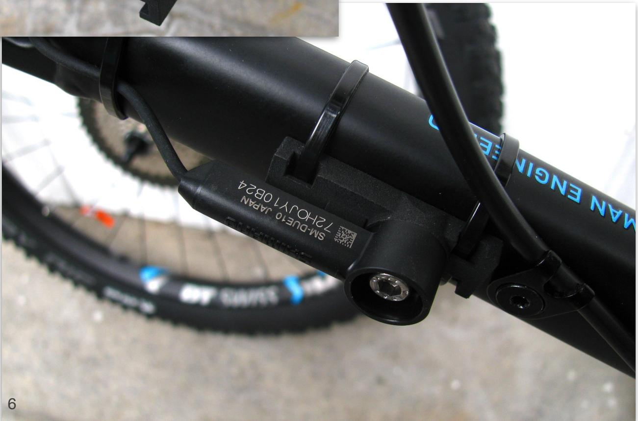
5. Screw the sensor onto the adapter.
