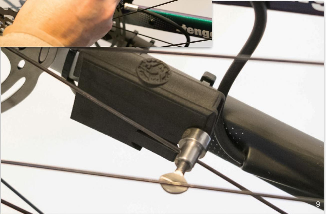
7. Slide the badassBox onto the adapter until it clicks into place. The badassBox is then upside down (which does not affect the function).
