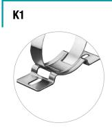
The **NORMACLAMP**<sup>®</sup> HMK K1 are prefabricated brackets which you can use to transform **NORMACLAMP**<sup>®</sup> standard clamps (types GBS, HD, SP and TORRO) into retaining clamps with brackets in no time at all. Just open the standard clamp, guide the band through the bracket slot, and that's all there is to it.
