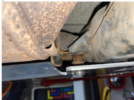
Is the protection kit right adjust, please drill the hole with a first step drill (4 mm) hole for the retract nut.
