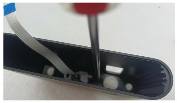
2. After fixing the panel, you can insert the motherboard into the housing and plug the cable
