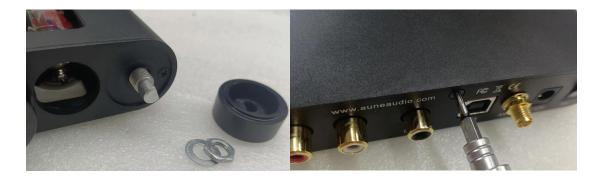
2. Pull out the Bluetooth antenna with one hand or carefully remove the rear board with pointed tweezers. Then push the potentiometer inward with one finger and pull out 1/3 of the motherboard with the USB holder in the other hand. Do not pull out all the motherboards as it is easy to damage the cable .
