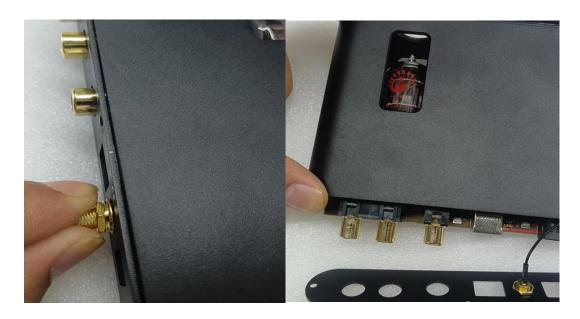
3. Use pointed tweezers to pull up the clips at both ends of the cable base, remove the cable and take out the motherboard to repair and replace the tube .
