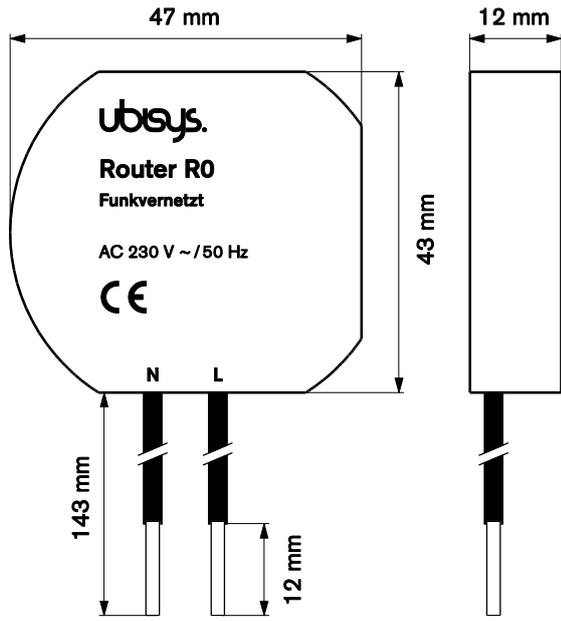
Figure 1: Flush-mounted In-wall ZigBee Router R0 – Dimensions
