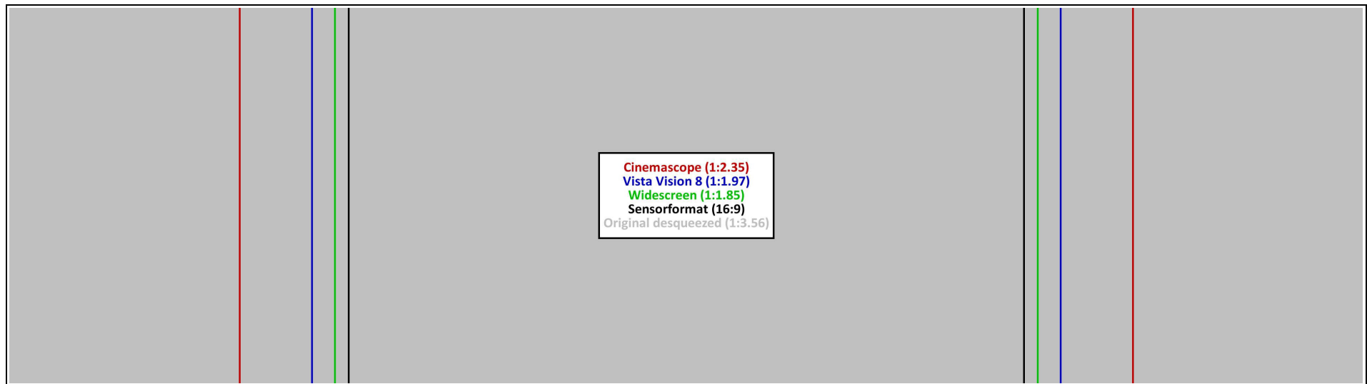
Illustration 33: Reframing - Sensors with Aspect Ratio 16:9 and Anamorphic Lens (2x)
