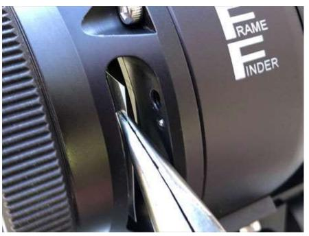
Then, looking into the front of the finder, center the frame-line pattern, left to right, and and top to bottom, and adjust any slight rotation if necessary, occasionally checking the alignment by looking into the eyepiece. Once aligned, tighten the four Phillips-head screws in the corners of the frame.
