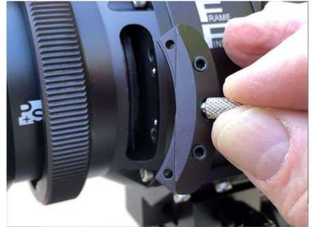
Remove the Lens Mount from the front of the Finder, by loosening the Neutral Mount Lock Ring. As seen from looking into the front of the finder, the plastic sheet needs to be oriented with the words at the top, and reversed, as shown in this photo. Also, note the four small Phillips-head screws in the corners of the rectangular plastic sheet retaining frame.
