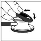
To assemble the nonchill bell sleeve, place one side of the sleeve on the edge of the chestpiece and stretch it over and around the chestpiece edge.
