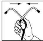
To increase the spring tension in the headset, squeeze the eartubes together. Repeat until the desired tension is achieved.
