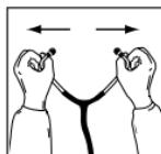
To reduce the spring tension in the headset, pull the eartubes apart. Repeat until the desired tension is achieved.
