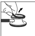
To remove the Littmann tunable diaphragm, pinch the rim of the diaphragm with your thumb and index fingernails; pull and lift the diaphragm from the chestpiece.
