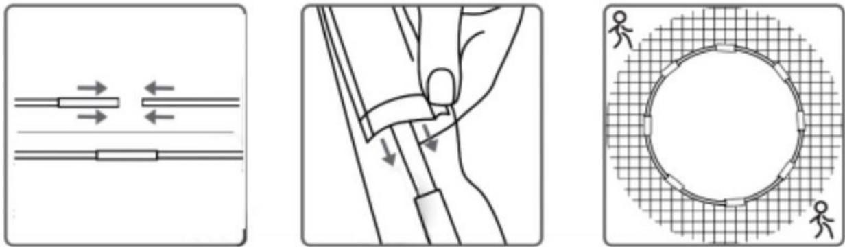
Attach the fiber rod to the frame by inserting it into the opening of the plastic cap and letting it click into place.
