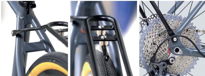
The FAHRER double rack is suitable for mounting on the usual fastening points on bicycles. M5 threads on the dropouts as well as threads on the rear strut or holes on the brake bar are required to support the strut.
