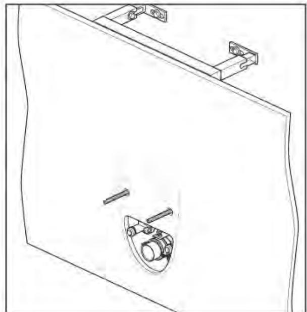
Build the partition wall, making the holes for the bolts and pipes. If required, tile the surface or apply the finish now.
