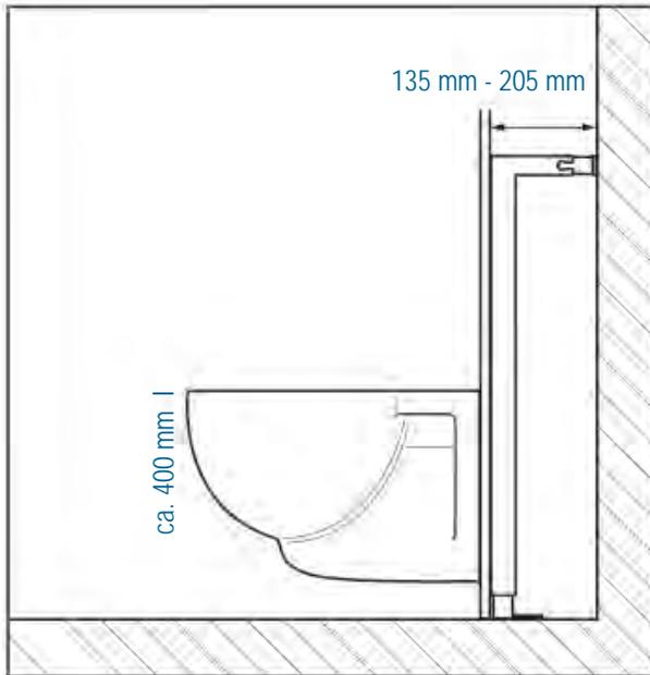
Plan the position of the bidet. The recommended bidet height is 400mm to the front rim. The maximum height will depend on the bidet that is used and the end users requirements. The distance from the wall may depend on the space requirements for a cistern if a toilet is being installed in the same run.
