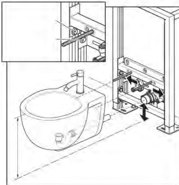
Carefully lift and position the bidet onto the bidet fixing bolts. Loosen the bidet support bar bolts and set the bar to the required height. Loosen the connection height adjustment bolts, set the connection support bar to the required height to line up with the waste outlet elbow. Retighten the bolts and remove the bidet.
