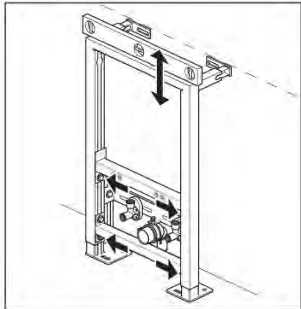
Place the frame against the wall in the required position. Loosen the height adjustment bolts (and bidet support height adjustment bolts), set to the required height, check the frame is level and retighten all 4 bolts.
