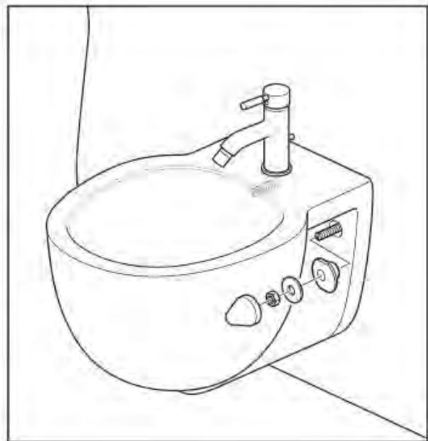
On each side of the bidet, place the plastic and metal washers onto the bolts, secure with the nuts and push fit the covers. Note: The bidet fixing bolts can be lengthened or shortened using a large flatblade screwdriver.
