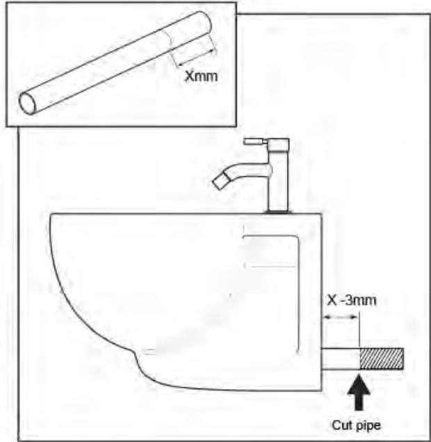
Measure the marked length of the 'spare' waste pipe (Xmm). This measurement MINUS 3mm is the length of waste pipe that is needed to extend from the back of the bidet into the waste elbow. Cut the waste pipe to length and remove any burrs.
