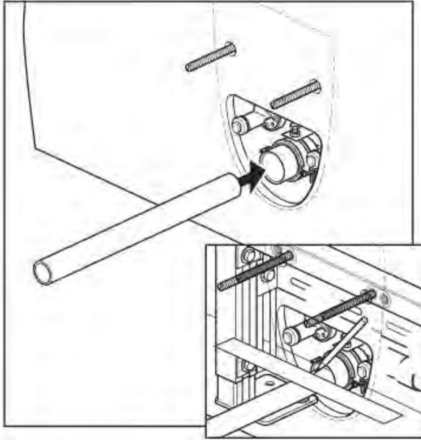
Push fit a 'spare' section of waste pipe fully into the waste outlet elbow.
