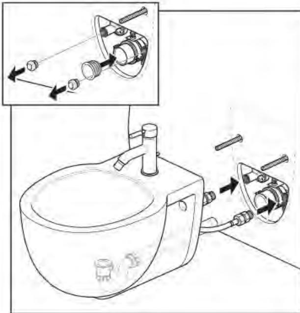
Remove the blanking plugs from the outlets. Push fit the waste pipe seal into the waste outlet elbow and lubricate the inside.
