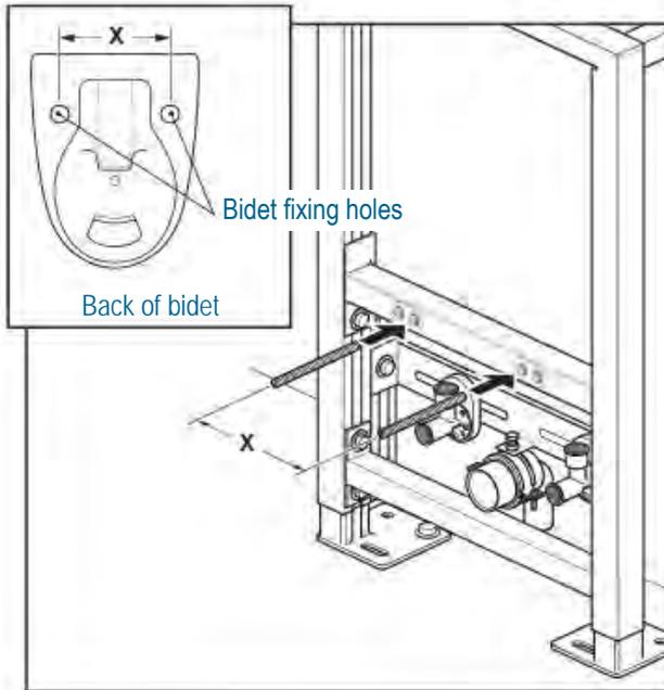
Measure the distance 'X' between the centres of the bidet fixing holes. Insert the bidet fixing bolts into the holes in the bidet support bar that match the bidet fixing holes. The fixing bolts can be adjusted (in or out) using a large screwdriver.
