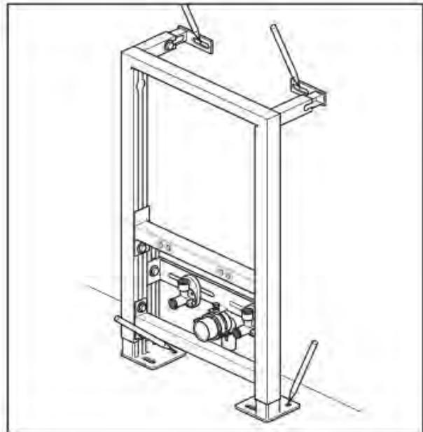
Mark the fixing positions on the wall and floor. Remove the frame and drill suitable holes for the fixings. Attach the frame to the wall and floor using suitable fixings. Check the frame is level in all directions.
