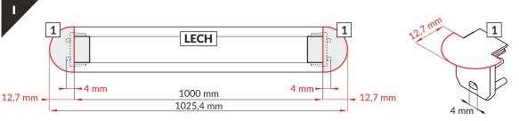
Note! Ending thickness increases the length of the luminaire (+ 2 x 12,7 mm) and the length of the mounting space (+ 2 x 4 mm).
