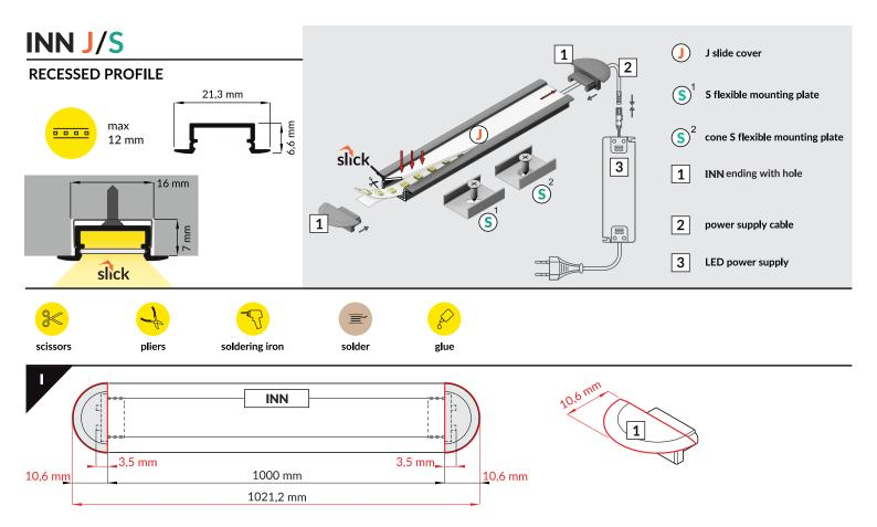
Note! Ending thickness increases the length of the luminaire (+ 2 x 10,6 mm) and the length of the mounting space (+ 2 x 3,5 mm).
