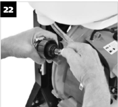
**EN** First loosen the hose clamp on the pressure cap nut on the right side of the spray tank. Then remove the nut and remove the hose.
