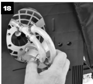
**EN** After removing the screws, remove the pump with hoses through the hole in the plastic frame (I).
