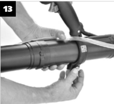
**EN** Adjust the control handle position (R) and secure it against further movement with the wing nut.
