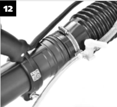
**EN** Insert the other end of the hose into the shut-off valve (M) and secure it with a clip.
