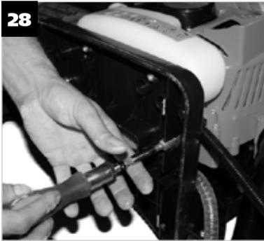
**EN** Place the the machine on its side, engine up, and remove two M6 nuts with washers and two M5 Allen screws with washers from the bottom with a spanner 10.
