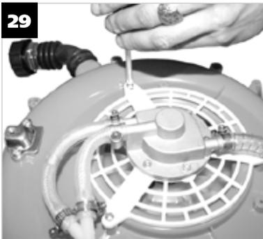
**EN** Remove the motor from the plastic frame and the pump grille.
