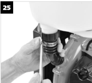
**EN** Refit the pressure cap nut and secure it with a hose clip.
