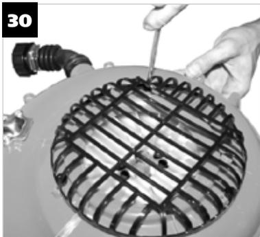
**EN** Attach the protective grille intended for permanent conversion, align the holes and fasten it with the screws removed.
