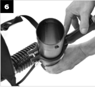
**EN** Slide the handle into the middle of the pipe, turn the handle by 90°, slide it into the groove on the shoulder and slide it to the end of the pipe.
