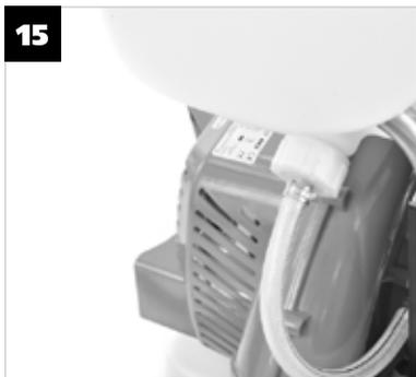
**EN** Remove the drain cap nut from the right side of the spray tank.
