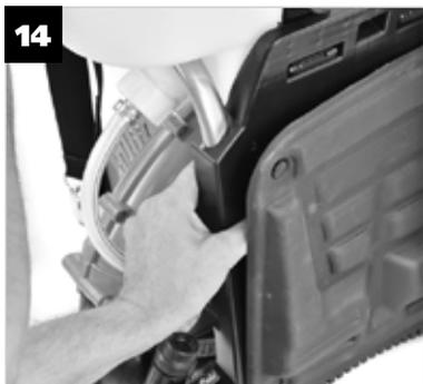
**EN Remove the spray attachment, disconnect the hoses from the shut-off valve. Remove the back padding.**
