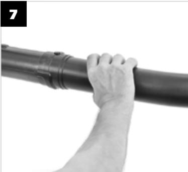
**EN** Connect the middle pipe (N) and the end pipe (O). Slide the protrusion on the middle tube into the fitting on the end tube, push the tubes together and turn them so that they lock together.
