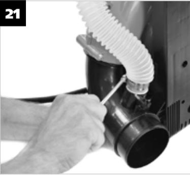
**EN** Remove the rubber plug from the bulk supply flap mounting and slide the free end of the flexible hose onto it. Secure the hose with a hose clip. (Open the inlet flap before mounting.)
