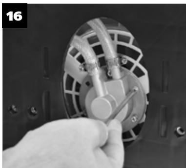
**EN** On the pump, loosen and remove the three pan head screws located on the spokes of the cover grille.
