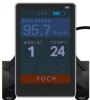
On the primary interface, long press the **Up** key to switch Day/Night mode. The background tune of the LCD display will shift.
