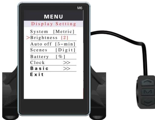
3) Short press the **M** key and the parameter will turn red for adjustment. Short press the **Up** key and **Down** key to change the parameter. Again short press the **M** key to exit the current setting mode, and enter parameter shift/choose mode. Short press the **Up** key and **Down** key to scroll the current chosen parameter.
